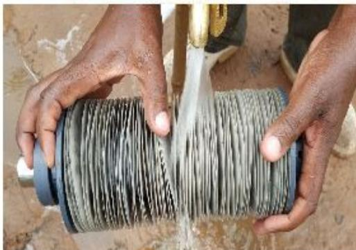
7) Please do not clean the filter with a solid object. Only by hand rinse down with clean water
