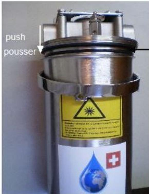
Clean the O-ring and push both parts together.
